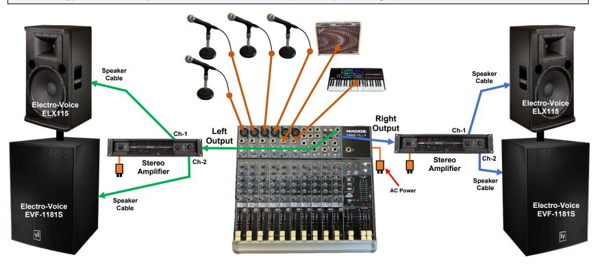
The diagram above is a "basic" version of a "Passive" speaker system set-up (example using speakers that have built-in crossovers). Usually, the output of the Mixing Board would first go to an Equalizer and / or a Compressor Limiter (or some other sound processing gear). The output from the "last device" would then feed the power amplifiers. This is just one example of a basic Passive Sound System set-up with the mixing board feeding the power amplifiers directly.
