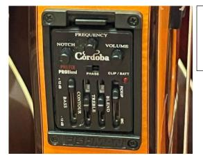
Typical Acoustic-Electric "Control" panel.
