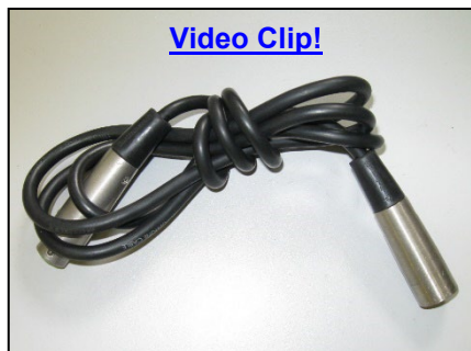
a) Wrong way to wrap a cable!
