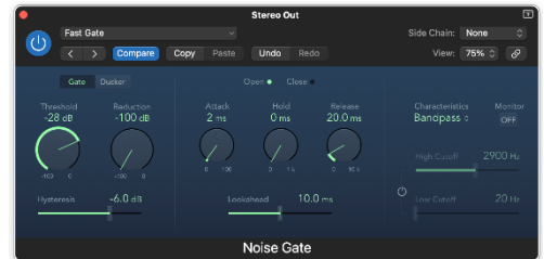
This is a screenshot example of a Noise Gate used in the Apple DAW “Logic Pro”
