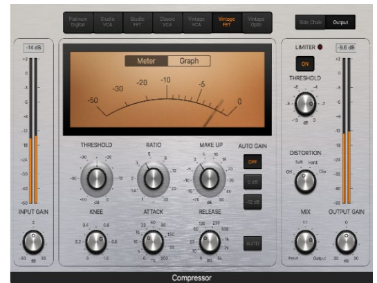
This is a “Digital” Compressor / Limiter used in the Apple DAW “Logic Pro”
