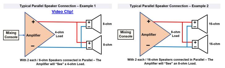
Example 1: If your power amplifier is rated at 4-ohms per channel, then you can parallel 2 each / 8-ohm speakers on each channel.
