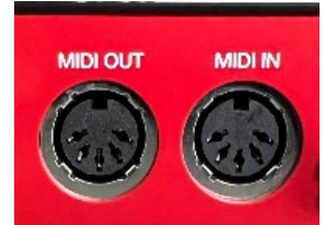
MIDI OUT / MIDI IN on the back of the MIDI keyboard shown left.
