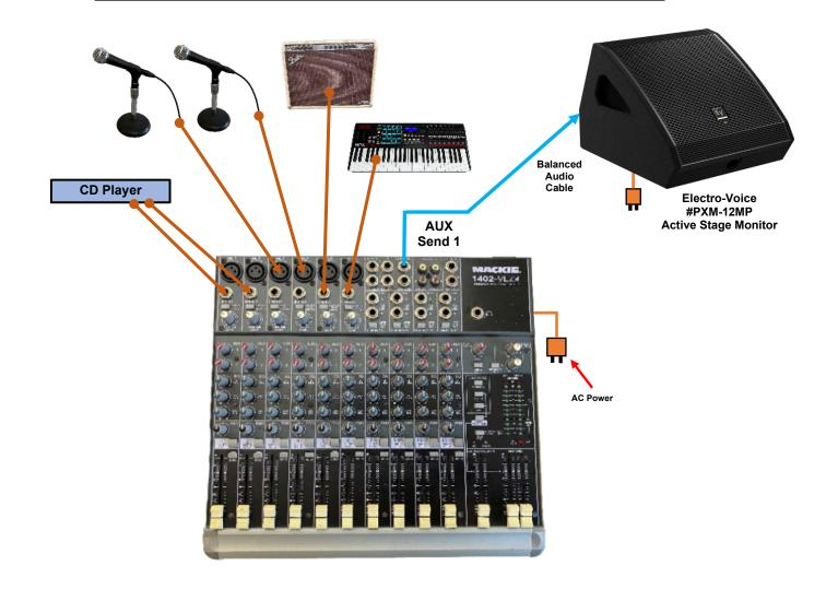
Typical Stage PA Set-Up – Example 2: Using "Passive" Speakers and Monitors with Built-In "Passive" Crossovers
